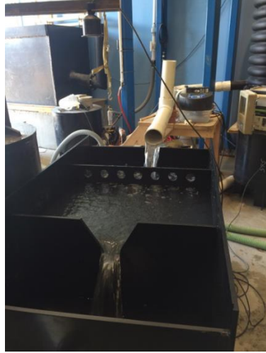
Figure 8 Photo of the Flow-Measurement System. The v-notch weir is in the foreground, with the ultrasonic sensor mounted above and slightly left-of-center in the photograph
