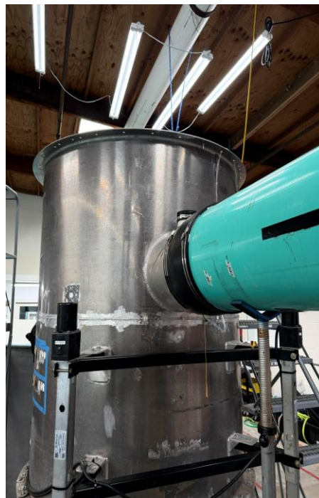
Figure 3: 5 ft. Diameter Test Unit
