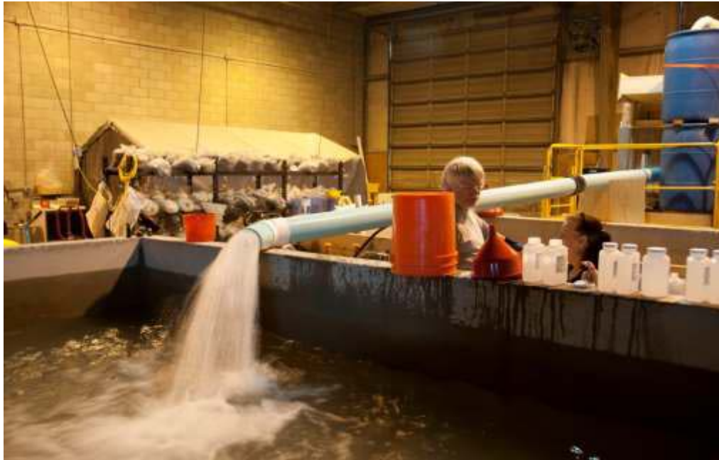
Figure 6 Effluent Pipe Discharging Water during Scour Testing
