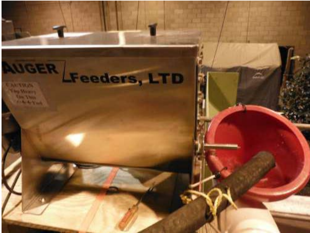
Figure 3 Vibratory Hopper, Mixing Funnel and Influent Water Line
