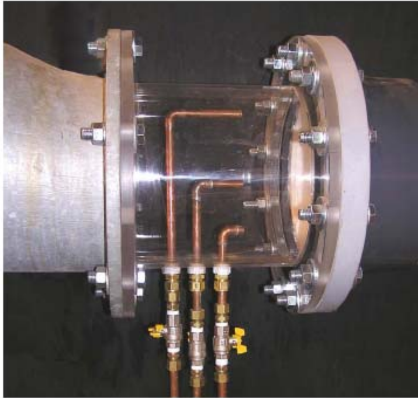
Figure 7. Photograph of Influent Sampling Tube Array
