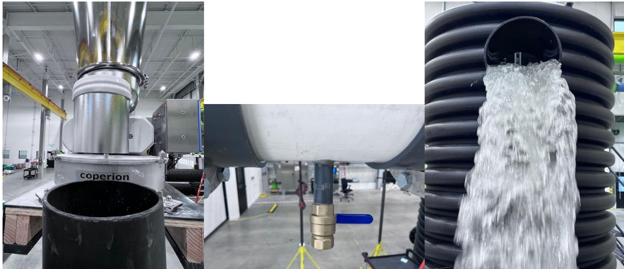
Figure 5 Arcadia ARC4 Test Unit Effluent Sampling Area, Sediment Dosing Port, and Background Sampling Area
