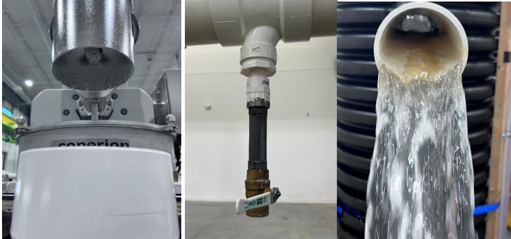
Figure 4: ALUX-3M Test Unit Sediment Dosing Port, Background Sampling Point, and Effluent Sampling Point
