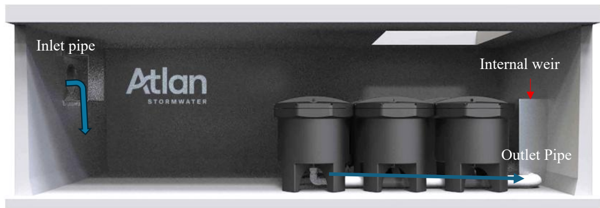
Figure 2. Typical AtlanFilter Arrangement (ATLAN Stormwater, 2025)
