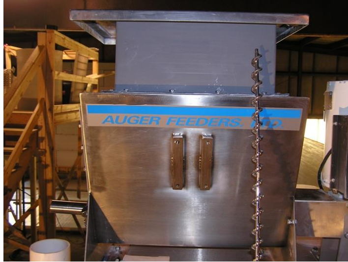
Figure 8 Photograph Showing Variable-Speed Auger Feeder
