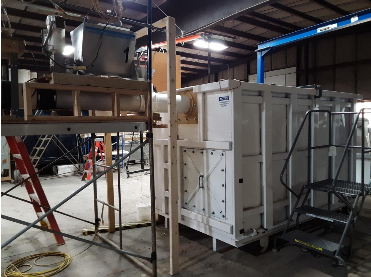
Figure 4 BioSTORM 0.5 Test Unit Installed in Alden Flow Loop
