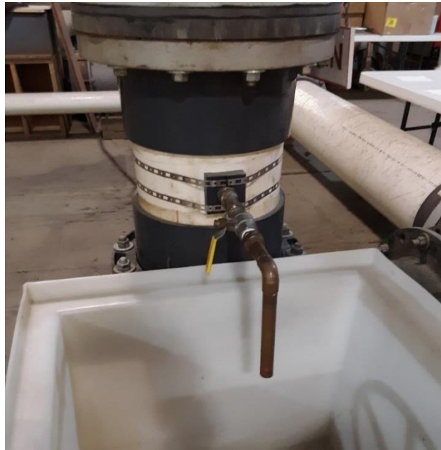
Figure 9 Photograph Showing the Background Isokinetic Sampler
