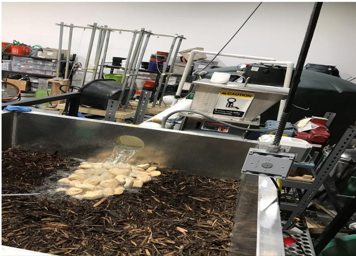
Figure 5: Photo of the Filterra HC Test Unit and Upstream Test Loop in Operation
