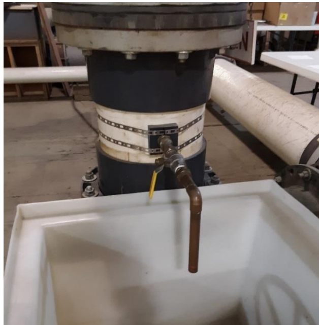
Figure 10 Photograph Showing the Background Isokinetic Sampler
