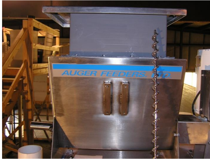
Figure 9 Photograph Showing Variable-Speed Auger Feeder
