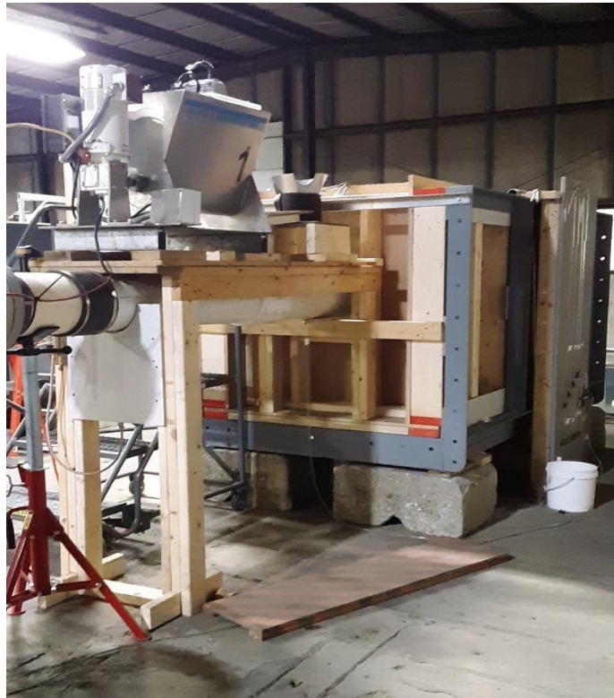
Figure 4 DryScreen ® Test Unit Installed in Alden Flow Loop
