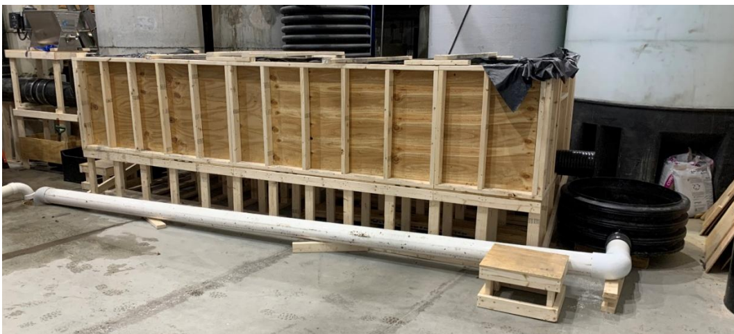
Figure 6 Side View Photograph of Isolator Row PLUS Test Box
