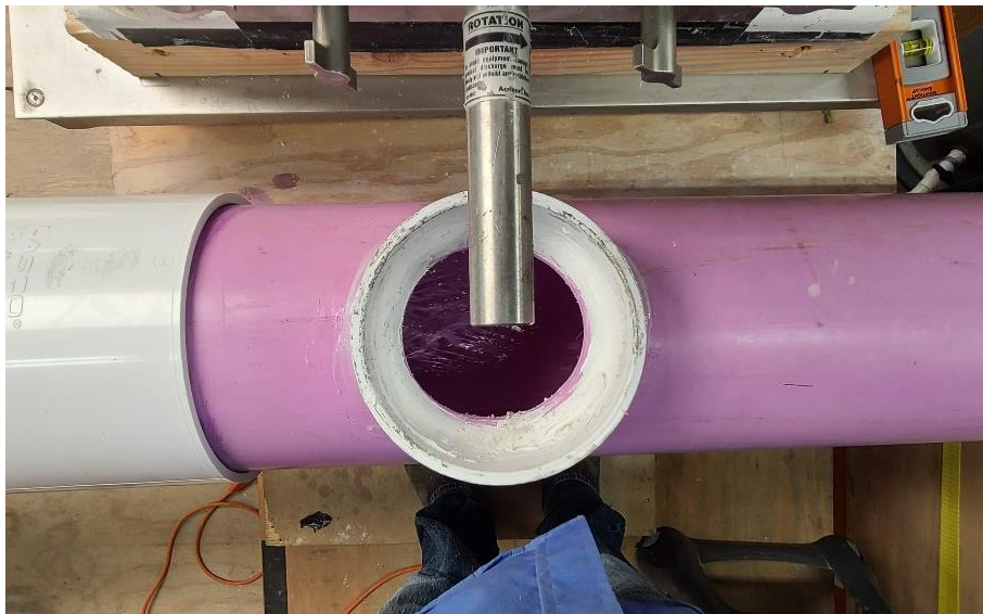
Figure 10 Sediment Injection and Sampling Point
