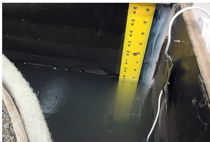
Figure 11 Water Surface Elevation Reading and Temperature Sensor Location
