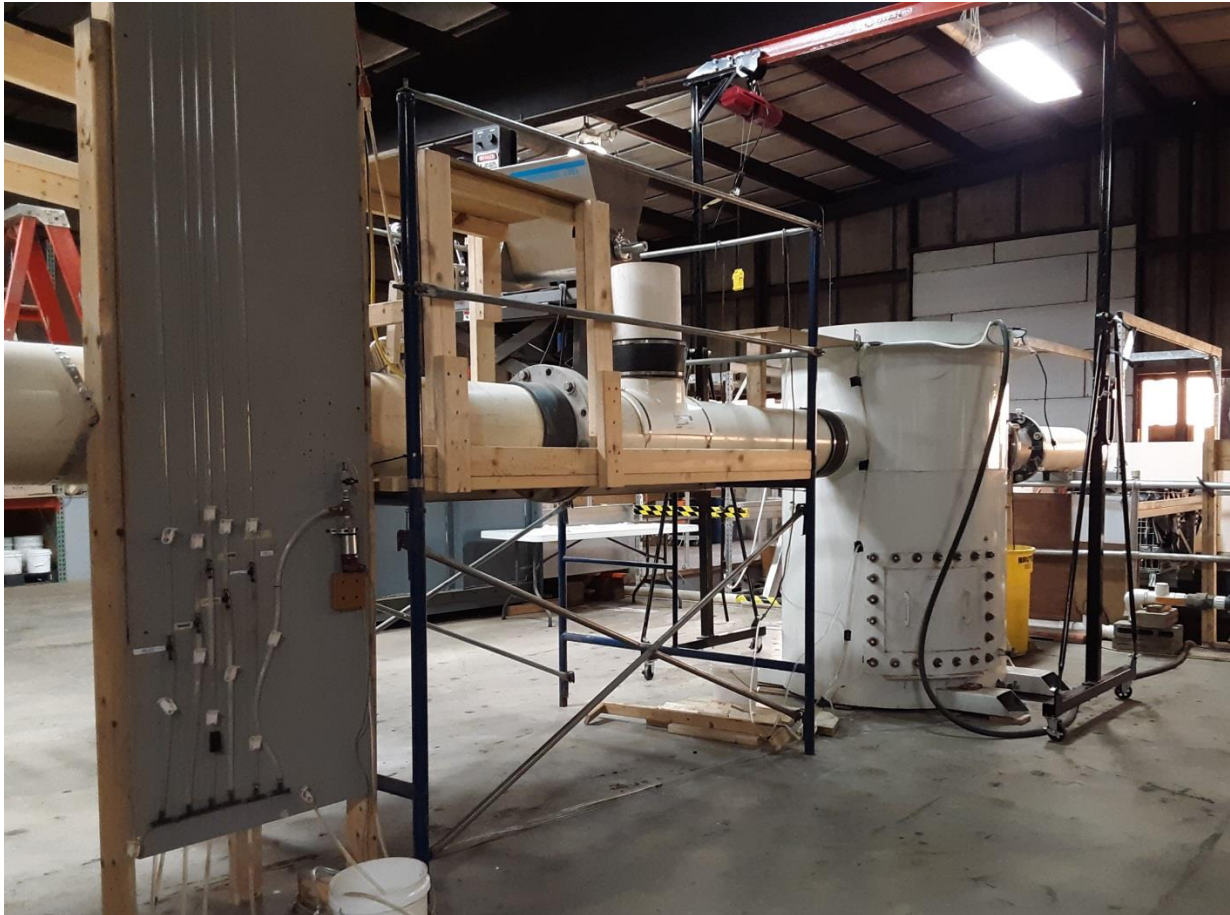
Figure 3 OG-48 Test Unit Installed in Alden Flow Loop
