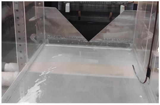
Figure 7 Effluent Channel V-notch Weir
