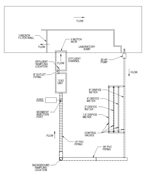
Figure 4 Alden's Stormwater Test Loop
