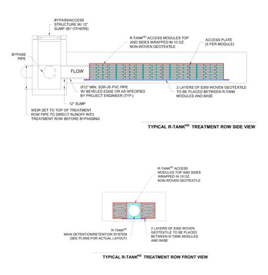
Figure 3 Typical R-Tank Treatment Row Section
