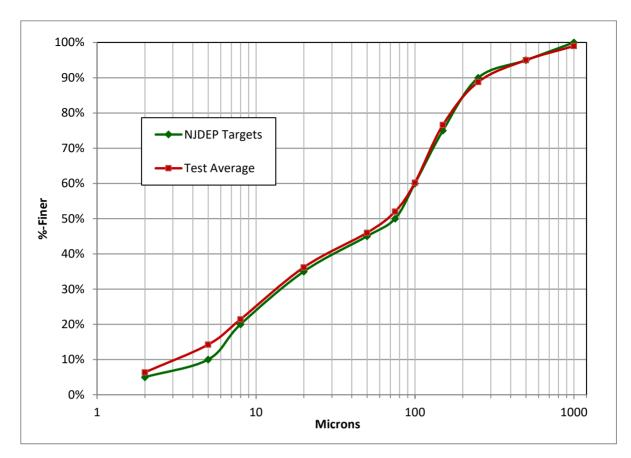
Figure 8 PSD Curves of 1-1000 micron Test Sediment
