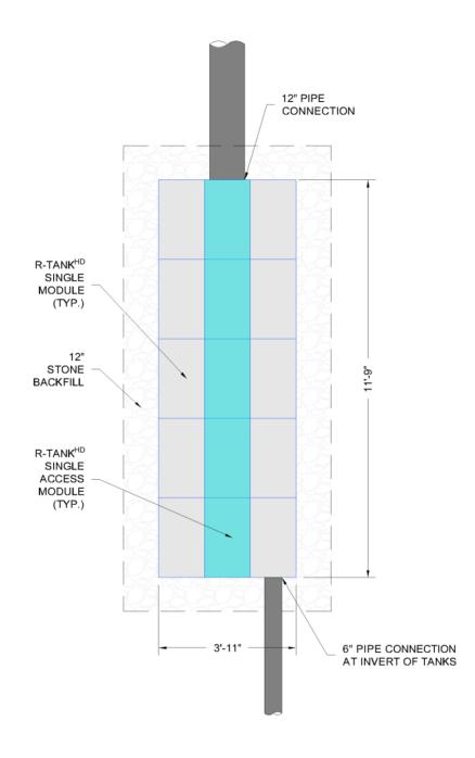
Figure 2 R-Tank Treatment Row Test Setup Plan View
