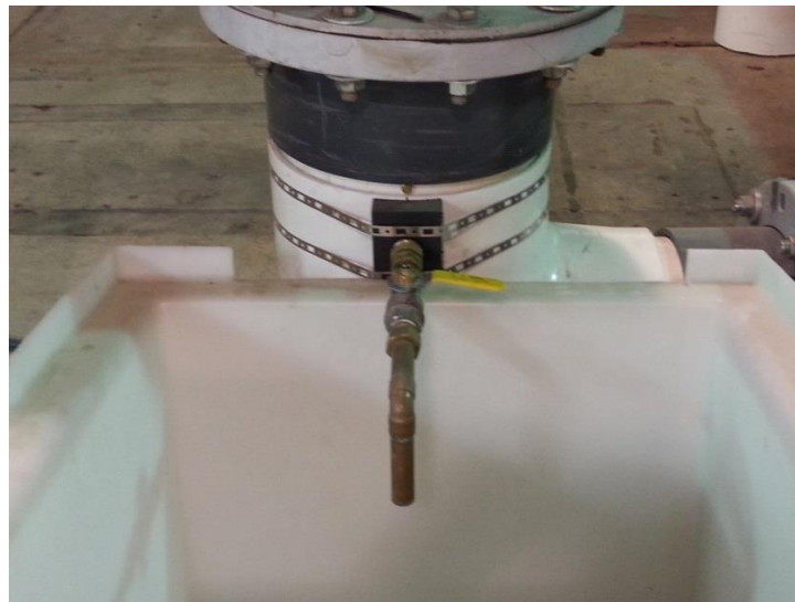
Figure 11 Photograph of the Background Isokinetic Sampler
