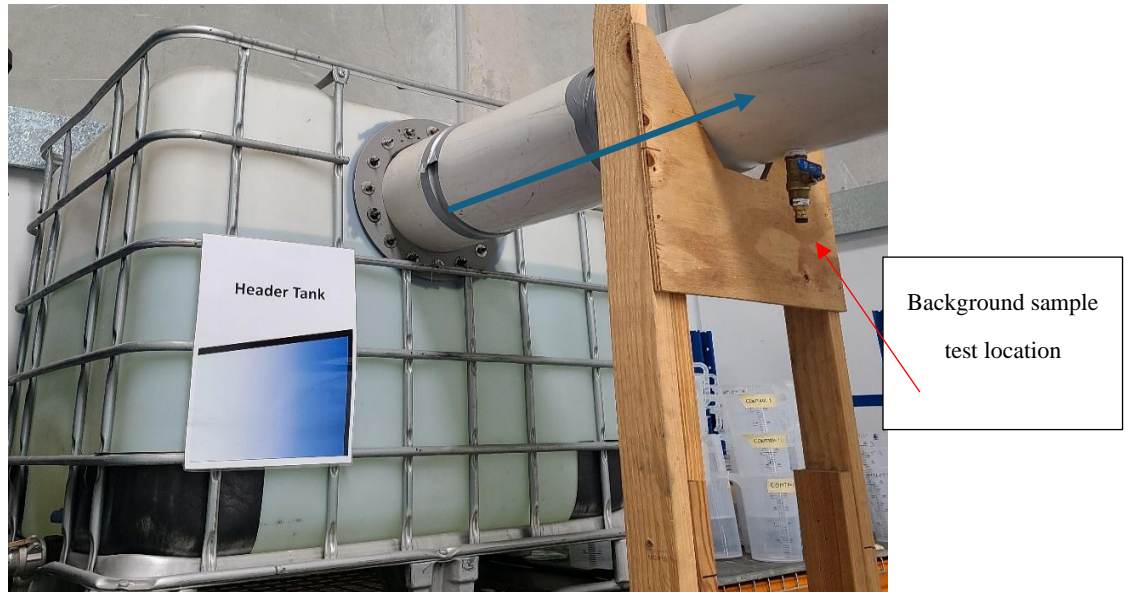
Figure 6 Photo of the Installed Constant Head Tank
