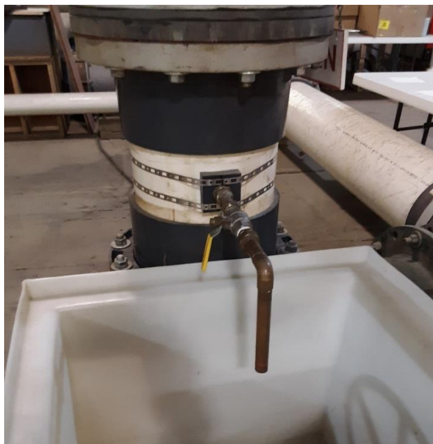
Figure 8 Photograph Showing the Background Isokinetic Sampler
