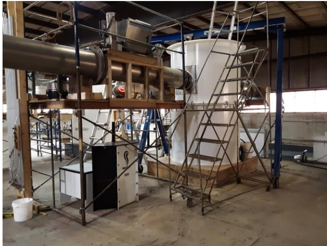
Figure 3 SAFL Baffle Test Unit Installed in Alden Flow Loop
