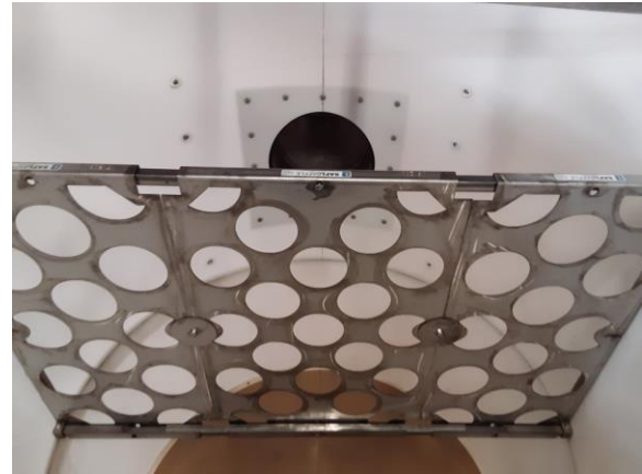
Figure 3 SAFL Baffle Test Unit Installed in Alden Flow Loop
