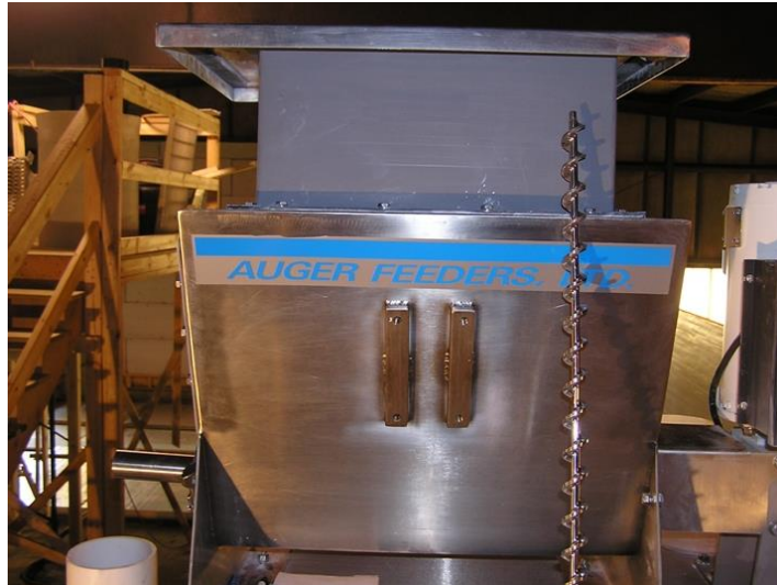
Figure 7 Photograph Showing Variable-Speed Auger Feeder
