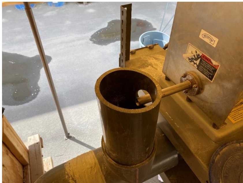
Figure 8 Vibra Screw Sediment Feeder with Windshield
