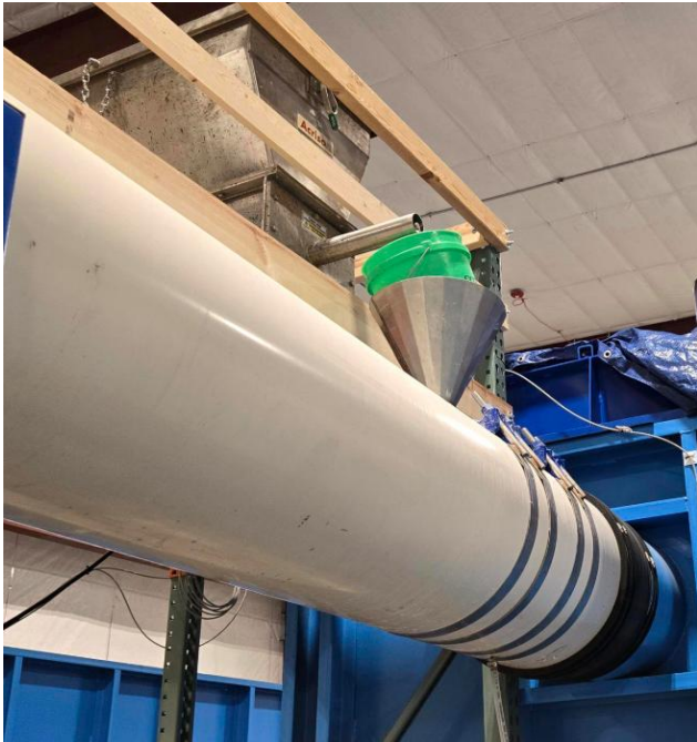
Figure 6 - Sediment Addition Port
