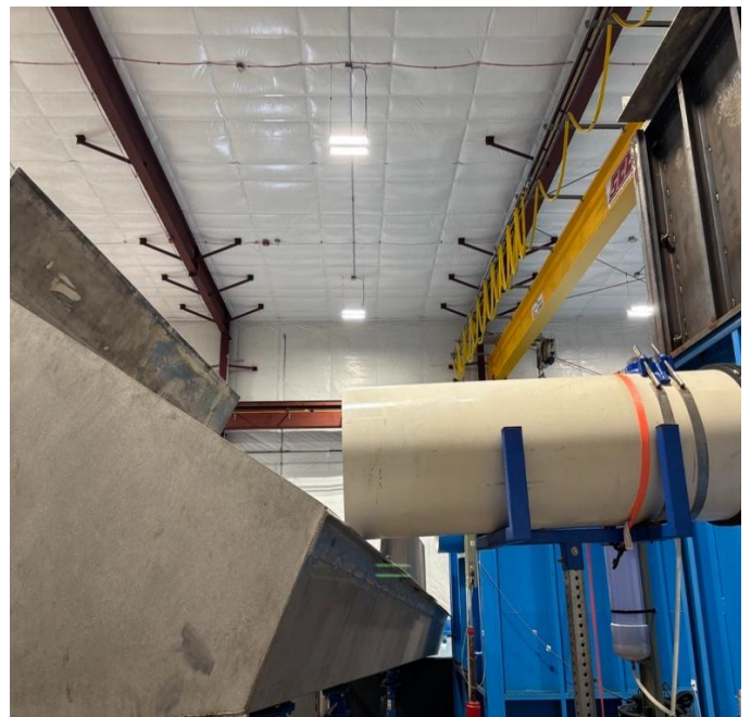
Figure 16 - Outlet Pipe and Effluent Return Channel Test Loop 3
