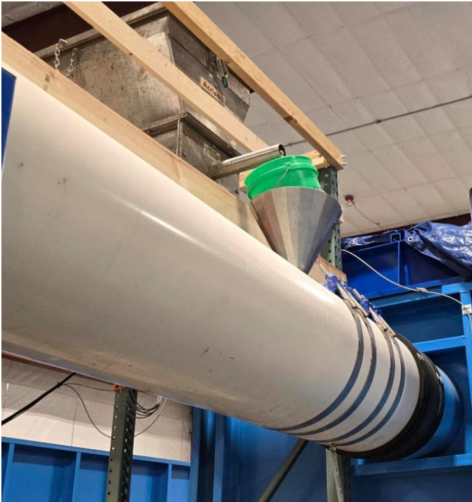
Figure 7 - Sediment Addition Port Loop 1 and 2
