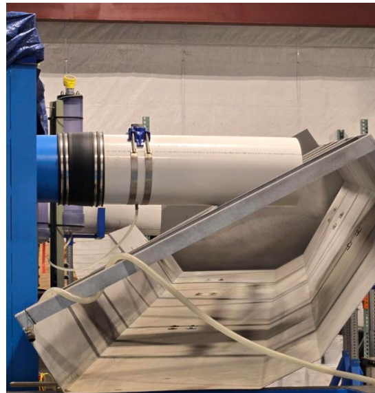
Figure 10 - Outlet Pipe and Effluent Return Channel Test Loop 1 and 2
