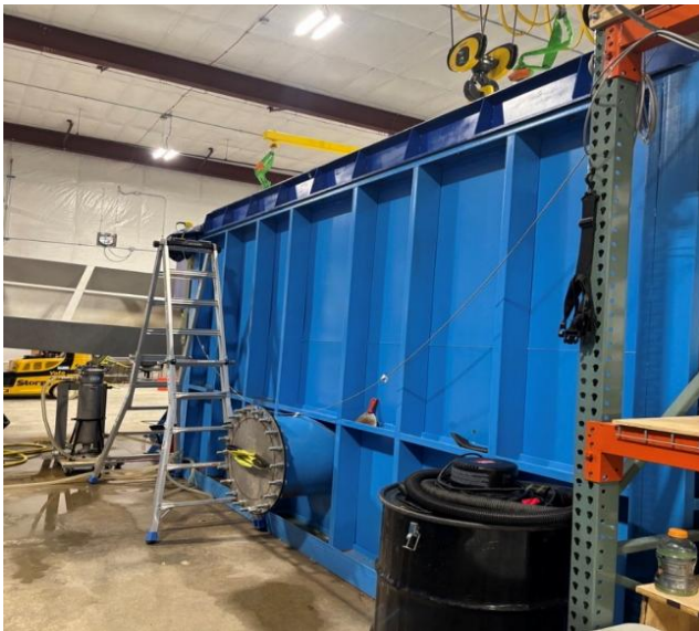
Figure 9 - SurgeSettler Unit and Access Port Test Loop 1 and 2
