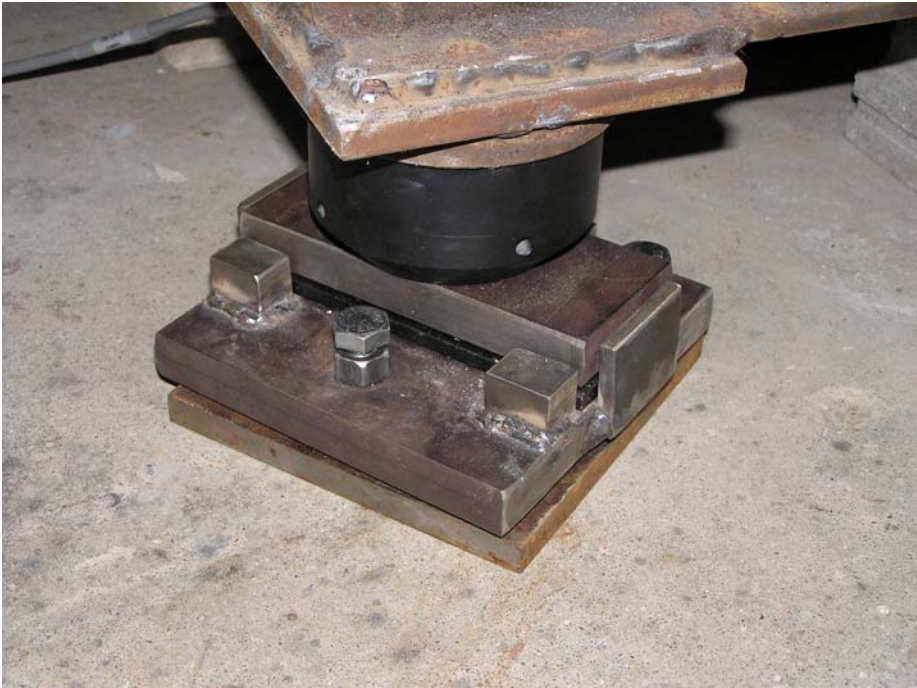
Figure 5 Load cell mounted on a transfer plate
