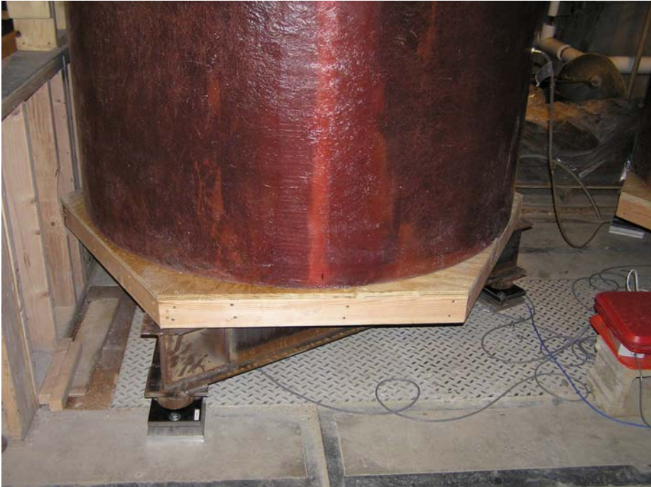
Figure 4 Support system of the M2 manhole
