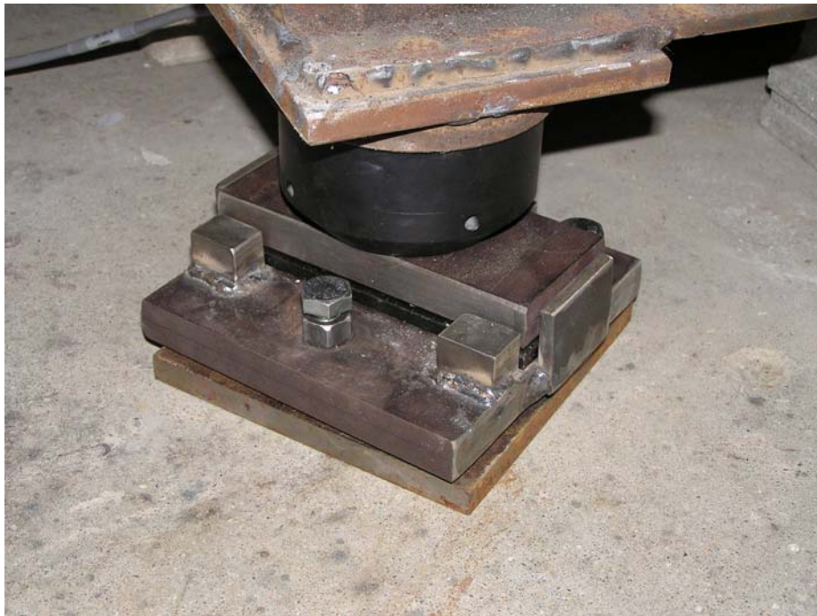
Figure 5 Load cell mounted on a transfer plate
